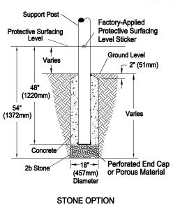
Support Post Factory-Applied Protective Surfacing Protective Surfacing Level Sticker **Ground Level** Varies - 2" (51mm) (1220mm) 54" (1372mm) Concrete Block <del>--</del>18"--**Porous** (457mm) Material
